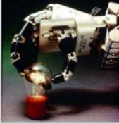
**Utah/MIT Robotic Hand** As a Visiting Scientist to MIT's Artificial Intelligence Lab, Dr. Gerpheide developed control algorithms to animate a dexterous robotic hand. With 16 degrees of freedom, this pneumatics actuated, tendon coupled, anthropomorphic hand can achieve most fine motor movements of the human hand.
